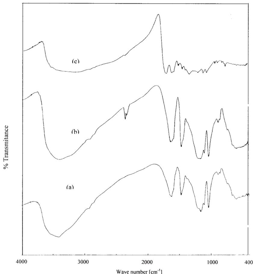
Figure 1 FTIR spectra of (a) PFR, (b) 10% (W/W) STCC in composite, and (c) pure STCC.
