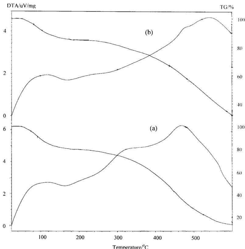
Figure 2 Thermal studies of (a) PFR, (b) 20% (W/W) STCC in composite.
