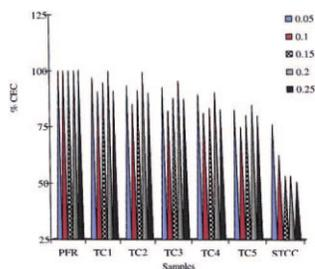
**Figure 5** Regeneration level for PFR, its composites, and STCC by using NaCl, after exchange with  $Mg^{2+}$  ions. [Color figure can be viewed in the online issue, which is available at [www.interscience.wiley.com](http://www.interscience.wiley.com).]
